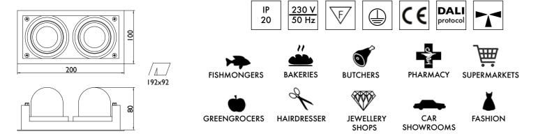
Recessed adjustable LED downlight. Body is made of die-cast aluminium and it is available in all RAL colours. Light source - Philips, Osram or Tridonic LED module. Standard EVG ballast, DALI or Touch Dali version on request. Passive cooling, optional IP44 diffuser and 3 hour emergency unit. Product is also available with special application LED modules: Crisp White, Food Warm White, Food Premium Red and many others - details on
