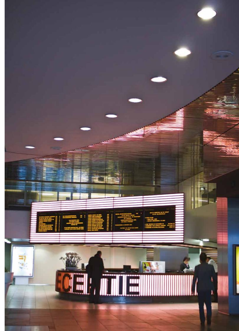
Recessed LED luminaire. Body is made of steel and aluminium and it is available in all RAL colours. Light source - Philips, Osram or Tridonic LED module. Standard EVG ballast, DALI or Touch Dali version on request. 3 hour emergency unit on request. This luminaire is also available with special accessory - additional ring which makes it semi-recessed. Opal diffuser can be mounted flat with the ring or recessed into the luminaire. High quality, energy efficient white LED light.
