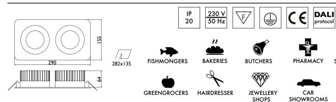
Recessed adjustable LED downlight. Body is made of steel and aluminium and it is available in all RAL colours. Light source - Philips, Osram or Tridonic LED module. Standard EVG ballast, DALI or Touch Dali version on request. Passive cooling, optional IP44 diffuser and 3 hour emergency unit.
